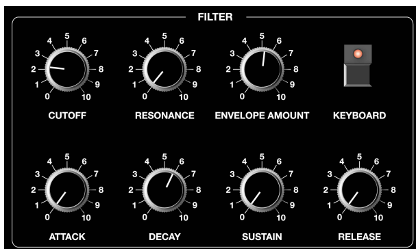
Figure 11: Using one of the Prophet 10's filters to create a far more accurate percussion sound.
