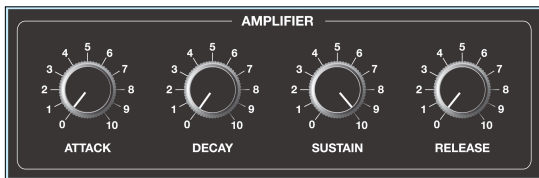
Figure 9: The 'organ' amplitude envelope settings.
